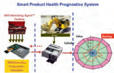
Figure 4: Machine health visualization using Watchdog Agent® technologies
